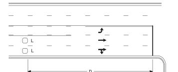
Speed Limit D D L = 6ft X 6ft Wired in series for Controllers
