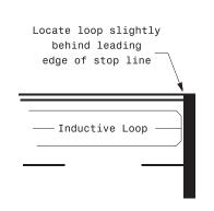
Loop may be located in advance of stop line under any of the
